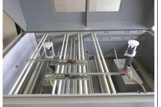
Res.6/Pic.6: Ray Korozyon Testi Rail Corrosion Test
