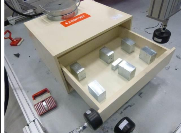
Res.5/Pic.5: Yatay Statik Yük Testi Horizontal Static Load Test
