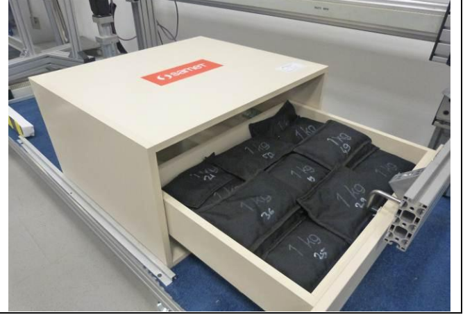
Res.2/Pic.2: Ray Açma - Kapama Dayanıklılık Testi 2 Rail Open - Close Durability Test 2
